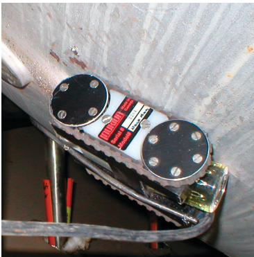
Vertical Inspection: Built-in rare earth magnets allow the Inuktun NanoMag™ to travel vertically, horizontally and even upside down on ferrous metal surfaces
