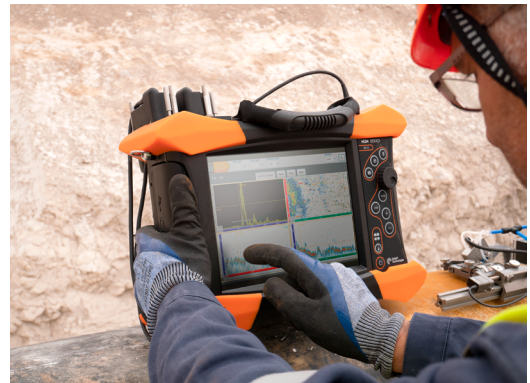
In-field inspection using M2M Gekko
